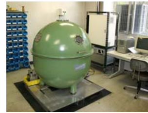
加工環境制御超精密加工機 (CAPSULE) Innovative mother machine for nano-machining
